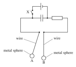
When the wires hang vertically the spheres are in contact and the discharging circuit is complete.
