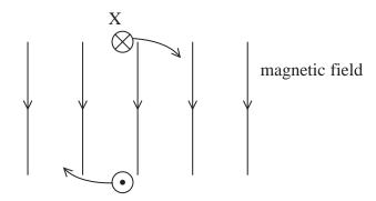
The coil is rotated clockwise in the magnetic field, causing a current in the coil. The student states that the current at X is into the page.
