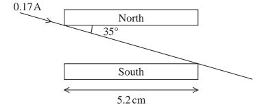
The magnetic flux density between the poles is 0.85 T.
